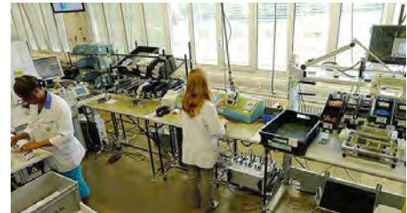
▲ Production cell for energy meters
