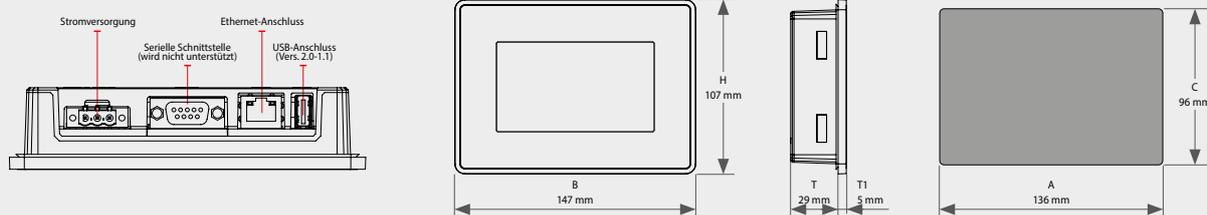
**PCD7.D570RF | 7" HTML5 Web Panel, resistive Touch-Bedienung**
