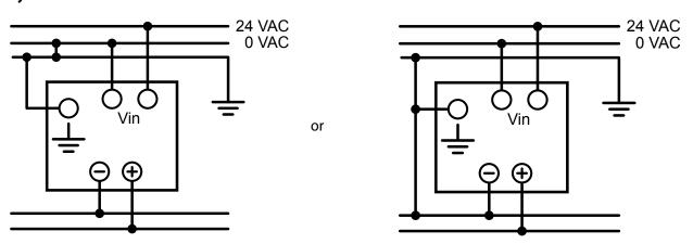
**Output:** Output voltage 24 VDC is made via the positive (+) and negative (-) terminals. The red LED DC signalises the correct output power. When the red LED is blinking, the device is in overload range or in short circuit protection.
