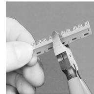
Cut the needed number of contacts with wire cutting pliers at the respective predetermined cutting point. Then insert the connecting bridge from the top into the contact slot and press it downwards into place.
