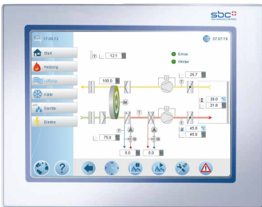
DDC Suite / HVAC templates created with Saia PG5® Web Editor 8
