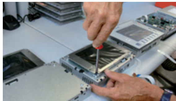
Manual assembly of panels
