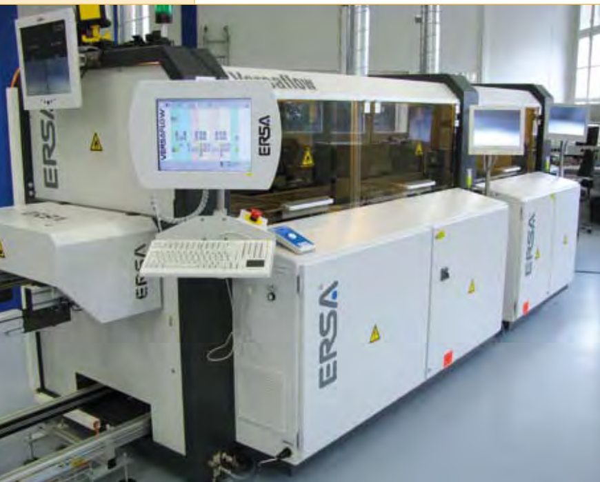
New selective soldering machine for Saia®PCD production
