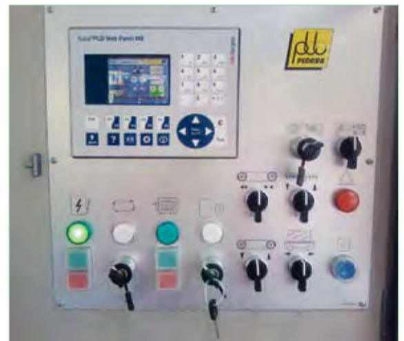
The operator interface of the new machine with 3.5" Saia® Web-Panel as central part.
