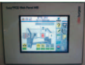
5.7" Saia®PCD Web-Panel MB. This Web-Panel allows the machine to be integrated into the company network
