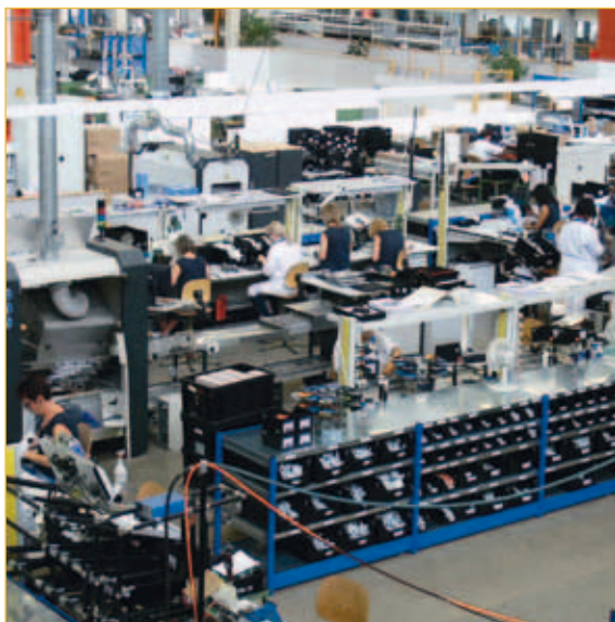
Assembly of energy meters and other control components as «lean production»
