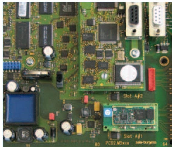
Saia®PCD7.F160S module in slot A of a Saia®PCD2.M5
