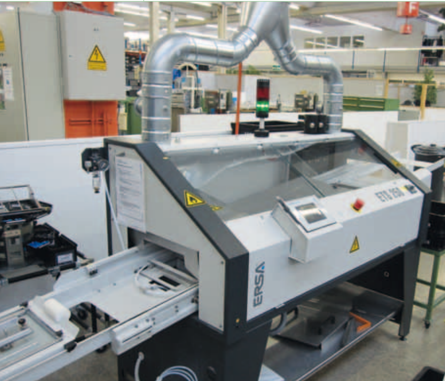
The new, small ERSA soldering machine with Saia®PCD2.M5 and 5.7" Web-Panel MB in the Saia-Burgess factory in Murten
