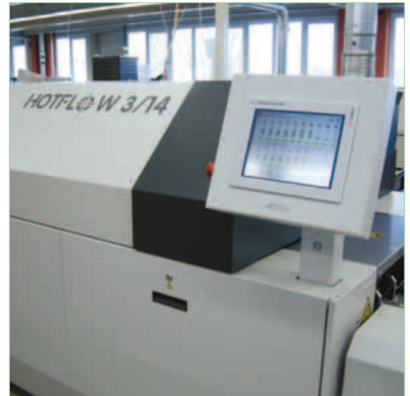
ERSA machine with Saia®PCD 10" Micro-Browser Web-Panel
