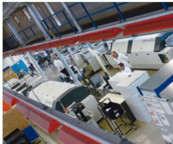
ERSA soldering machines, controlled with Saia®PCD, in the Saia-Burgess factory in Murten. Comfortable operation with Saia®PCD Web-Panels.
