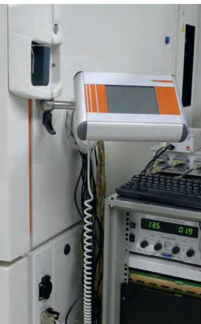
▲ Expensive assembly systems are required to be able to read the panel better to compensate for the «cheap» STN LCD technology. Now it is only in the way...
