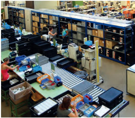
SBC Production before lean: Distributed units and lots of material in circulation = fragmentation of responsibility.
