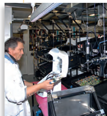
▲ System and energy manager assembly line for the Vaillant-Honda micro-CHP system: The SBC boards are assembled and tested according to lean methods on the production line created for this product
