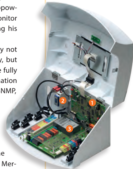
1 Standard SaiaPCD® CPU board 2 1-phase SBC energy meter 3 Vaillant-specific I/O board
