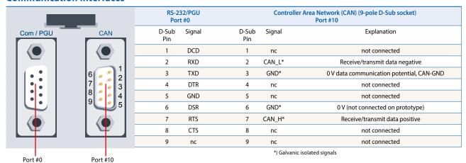
PCD3.M6240 CPUs provide a galvanic isolated high-speed 1 MBit/s CAN interface.
