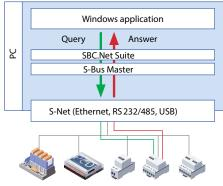
Automation devices Saia PCD® system (S-Bus Slave components)
