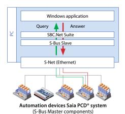
Native communications driver and .Net class libraries for efficient integration of S-Bus components into Windows® applications. By integrating the S-Bus slave component, the application can react to events and trigger the corresponding functions or answers. Since the Windows® application no longer has to poll individual stations, network load can be greatly reduced with S-Bus Slave.
