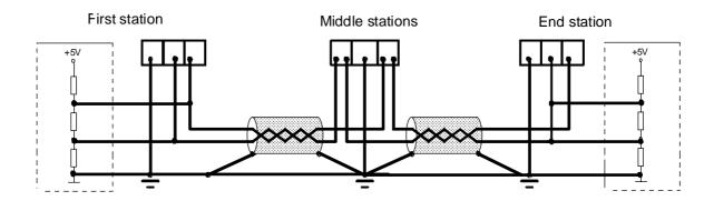
It is recommended that the RS 485 cable is not laid in direct proximity to motor cables which may be produce interference, unless these cables are also well screened.
