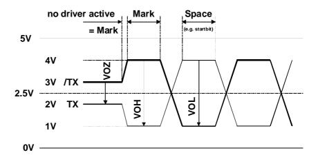
VOZ = 0,9V min... 1,7V max (no driver active) VOH = 2V min (with load) ... 5V max (without load)
