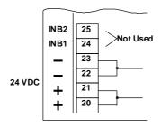
Connection takes place at plug-in terminals 20 to 23 with wires of max. 1.5 mm<sup>2</sup> (with cable end piece)
