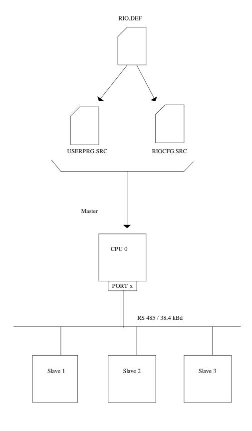
The following drawing shows the various files which must be linked and loaded if a PCD4.M445 is used as the master PCD (dual processor CPU).
