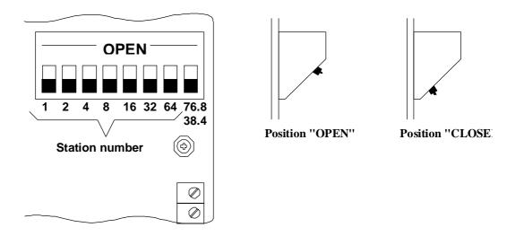
The 8-position DIL switch on the PCD1.RIO is used to configure the station number and transmission speed.
