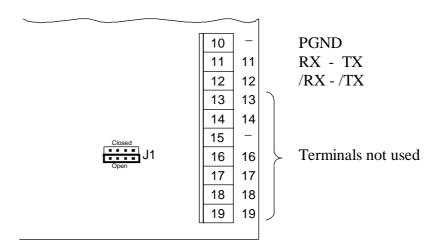
For the correct adjustment of line termination resistors (position of jumper J1: "open"  $\rightarrow$  without termination resistors) and the laying of the bus cable, consult the "Manual of the PCD2 series hardware", "SAIA® S-Bus manual" and "Installation components for RS 485 networks".
