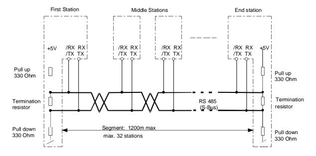
When using the internal resistors of the processor or bus modules to terminate the lines, these stations can not be powered down otherwise the communication over the network is no more possible.
