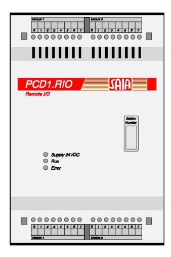
The PCD1.RIO includes an RS 485 interface for connection to the RIO network. An 8-position DIL switch enables the station number and transmission speed to be adjusted. The PCD1.RIO is not programmable. Once the PCD1.RIO has been configured, connected to a supply, linked to the RIO network, and the station address and transmission speed adjusted via the DIL switch, the device is operational and further handling is unnecessary.
