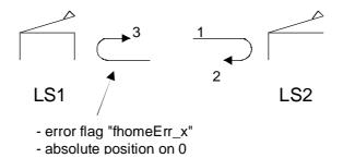
If FB 'Home' returns because the specified timeout has been exceeded, diagnostic register 'rDiag' is additionally loaded with code 9 as the parameter number (timeout is parameter 9).
