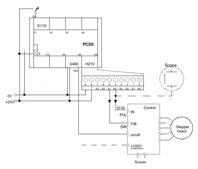
Minimum arrangement to operate a stepper motor for control using a PCD2.H210.
