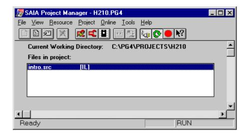
'Project' - 'Build' processes the program and downloads it to the PCD. Commissioning is done using the debugger.
