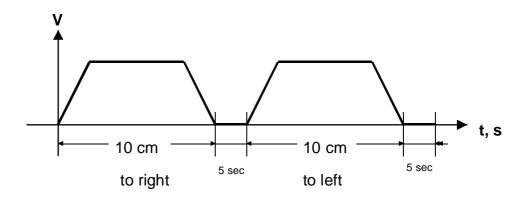
As a variation, the motion of the carriage is to be stopped with PCD input 1 ("Stop") and made to run on with PCD input 2 ("Continue"), retaining acceleration and braking ramps.
