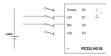
When "LS1" or "LS2" become active (voltage = 0, LED off), a braking ramp is triggered directly if the switches have been configured as limit switches.
