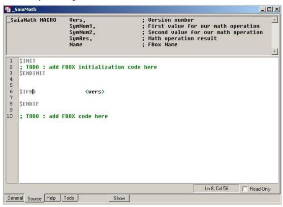
In the upper pan, you can see the macro header generated by the FBOX Builder. This part is read-only and it is entirely managed by the FBOX Builder. What you can see in this macro header:
