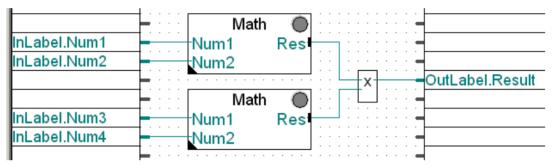
The Adjust dialog of each "Math" FBOX stays unchanged that means each "Math" FBOX does a simple addition between "Num1" and "Num2". The results of both of them are finally multiplied.
