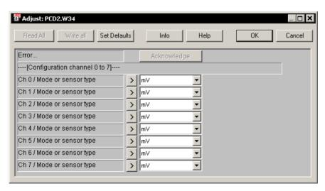
The structure of this dialog is defined by the AV entries of the definition file; but the text displayed are defined in the "FBOX Display Texts" (.IDX file) which we will see the details in the next paragraphs.
