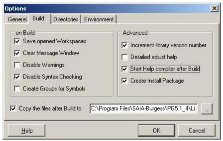
Before generating the files, you should select also the "Copy the files after Build to" and select the "Usr" directory of the PG5 library folder. If this option is not selected, you'll have to copy by hand all the generated files in this directory to be able to use your FBOX in FUPLA.
