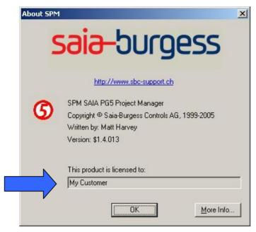
To install your Library, your customer will have to enter the generated key during the installation process. The installer will also enter a key in the computer registry of the customer, which will be used by PG5 to check the right to use this library.
