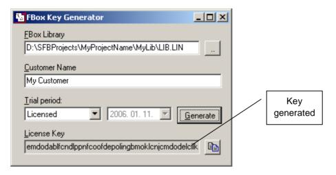
In the FBOX Library field should be filled by default if Key Generator is opened from FBOX Builder and it should display the full path of the LIN file of your active library. The path of this LIN file is the following:
