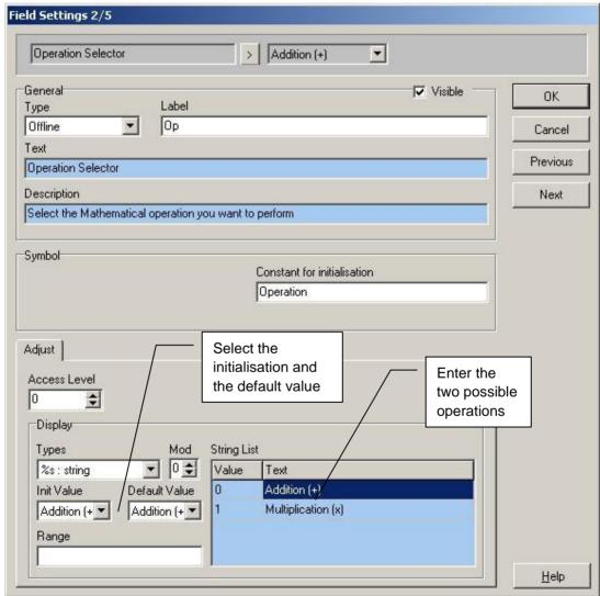
**Note:** If the string values are not continuous (e.g. 0, 1, 5, 6, 8) then Range field must be filled too, based on which item should be visible.
