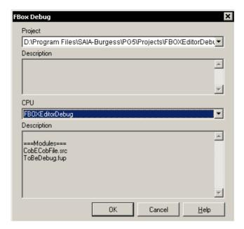
Click on the "OK" button, the FBOX Builder will start the PG5 to compile a first time the project, then the FBOX Builder will modify the "FBD" and start again the PG5 to recompile the project with the modified files. At the end of that process, you get this dialog:
