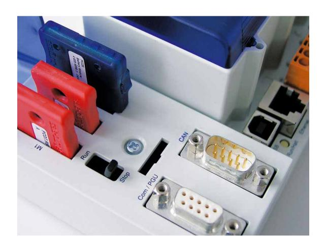
CAN-Functions on PCD2.M5\_ & PCD3
