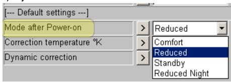
This can be useful if no timer clock is used for the changing of the operation mode.
