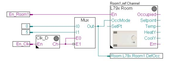
This can be useful if a timer clock or superior system is used for the changing of the operation mode.
