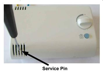
With a screwdriver (diameter less than 2 mm) the Service Pin can be activated
