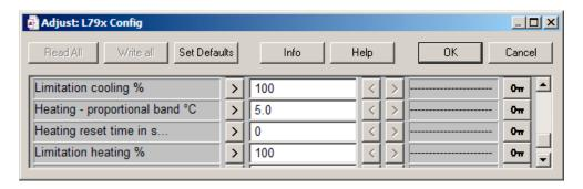
The current value is set in the Room FBox (register 142 for cooling and register 143 for heating)
