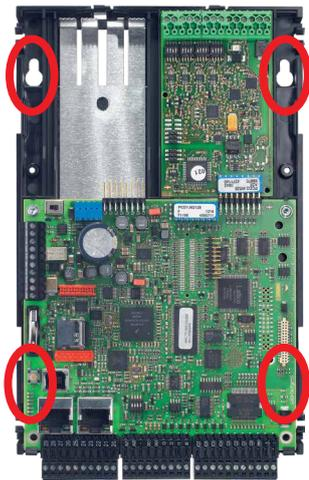
Two holes in the base plate for fastening the controller..
