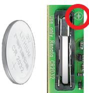
Insert the Renata CR 2032 button battery with the label side (+ pole) up, slightly pushing the battery retaining clip to the side.
