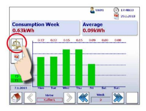
3. The reference bars are shown along with the name of the reference meter and the period at the top ritht of the screen.
