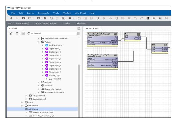
The **Out** pin of the And Function box must be connected to the Enable\_Light pin **IN16**. But these Function Boxes are located in two different Wire Sheets. We need to link these two pins together.
