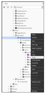
The not used "SBClpNetwork" then can be deleted.
