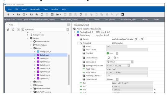
The same way it is possible to create every needed points and connect it to the corresponding media element of the SBC PCD device.
