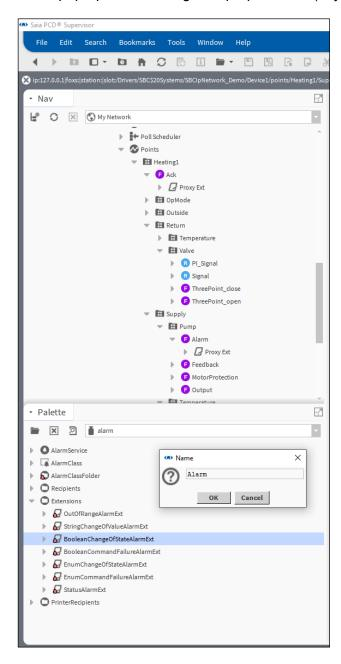
6. Set up the properties of the Alarm Extension
