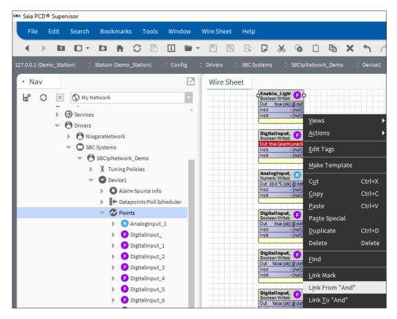
13. In the pop-up window the link between the two Function Boxes must be defined as the picture shows. The link can be checked by reading the text at the bottom left corner of the window.
