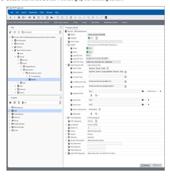
Setup the IP address and the S-Bus Station ID of the Device 1
