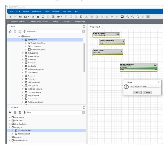
4. Wire the Alarm console and the Alarm Classes together as the next image shows. The system has to know what to do with the alarms so that the Alarm Classes (container of alarms) and the Alarm Console (a way to display them) has to be connected.
