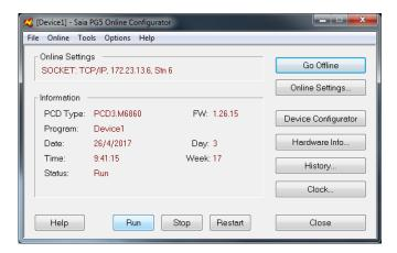
2. If it's not possible to go online over Socket to the PCD, try to ping the IP-address of the PCD.
