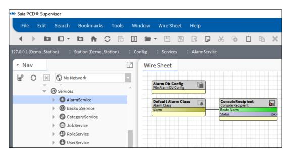
The default view (Wire Sheet) will be displayed with the default settings. (Alarm Db Config, Default Alarm Class and the Console Recipient).
