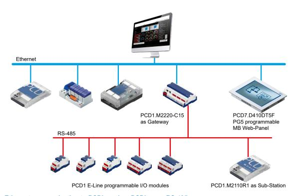
Ethernet communication to PCD's and on PCD's over RS-485 which are connected behind a gateway.
