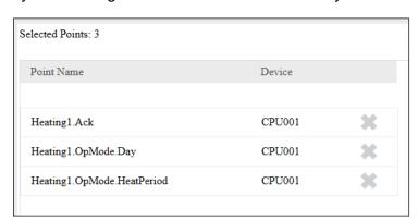
7. Because in the middle window of the wizard shows all the symbols the System integrator has to be able to select the symbols which are needed to be imported. Filter can be defined, so only the interesting symbols will be shown.
