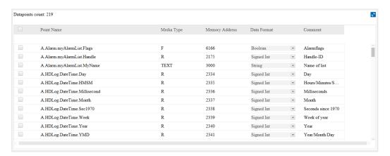
The symbols can be selected one by one by checking the checkbox beside the symbol. Or at the top beside the Point Name by checking the checkbox all the symbols are getting selected in the actual group.
