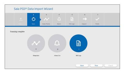
The detail view of the HD Logs is displayed. Select the needed HD Log files. Inside of one HD log file can be many different data points logged (symbols). Then press Next.
