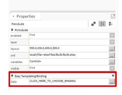
2. Using either the Properties Sidebar, or the Properties Popup (double click), there will be a Easy Templating Binding on the Simple Object with a property reading "CLICK\_HERE\_TO\_CHOOSE\_BINDING". Clicking this will bring up matching location which meet all the points used in the Simple Object.
