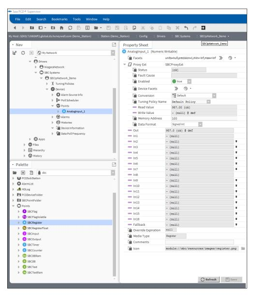
5. The Status must be **{ok}**. It can be seen that the "Read Value" and the "Out" are following the content of the "Device1/Register 100".
