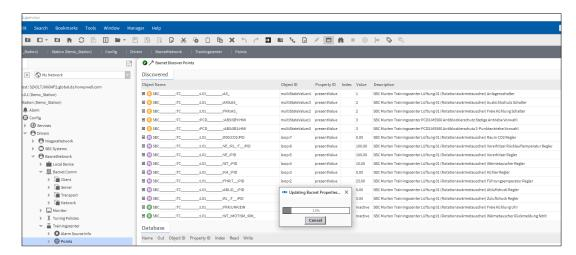
5. In the **Discovered** list select the required points (values). To select more than one point hold down the CTRL key and click on the required points.
