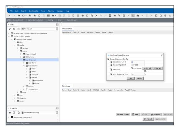
If the address range of controllers is known then the **Device Low Limit** and **Device High Limit** can be edited to reduce discovery time.
