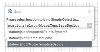
3. Once a selection has been made, the resources needed for the Simple Object will be copied over the from the Simple Object directory, into the running station. The variable will then be set, linking the graphic to the chosen location.
