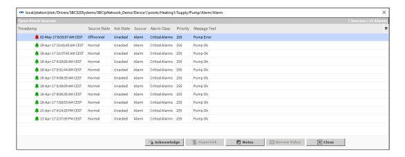
5. Double click an alarm to open the Alarm Record, giving full details of the alarm.
