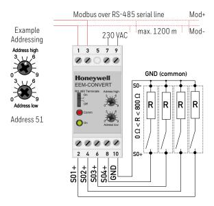
Note: If the SO-Modbus module is used in the Modbus as last device, then the sliding switch «RS-485 Terminate» need to be in the position «On».
