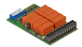
The module contains 8 relays with normally-open contacts for direct or alternating current up to 2 A, 48 VAC. The module is especially suited wherever AC switching circuits with infrequent switching have to be controlled. For space reasons, there is no integrated contact protection.
