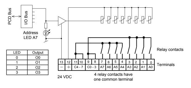
Relay energized (contact closed):LED onRelay reset (contact open):LED off24 VDC must be connected to the +/- terminals.
