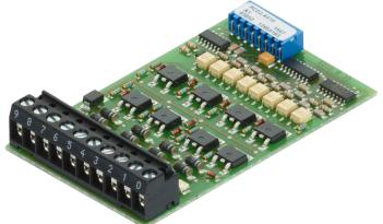
Output module, electrically isolated from the CPU, with 8 MOSFET transistor outputs, without short-circuit protection. Voltage range 5 ... 32 VDC.
