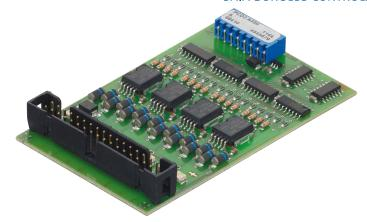
Low cost output module with 16 transistor outputs 5 ... 500 mA, with short-circuit protection. The individual circuits are electrically connected; the voltage range is 10 ... 32 VDC.
