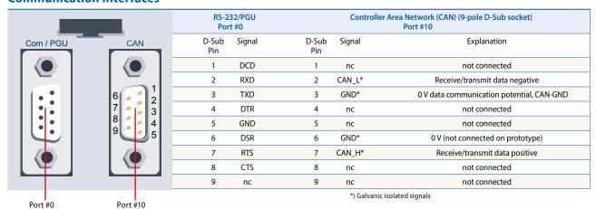
PCD3.M6340 CPUs provide a galvanic isolated high-speed 1 MBit/s CAN interface.
