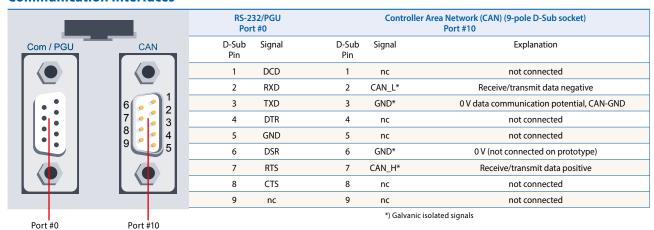
PCD3.M6360 CPUs provide a galvanic isolated high-speed 1 MBit/s CAN interface.
