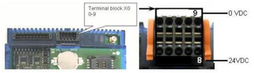
Terminal block X0, connector 8: 24 VDC for GSM Modem Terminal block X0, connector 9: 0 V GND for GSM Modem
