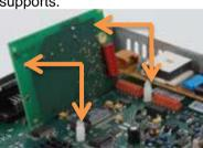
6. Module is installed. Make sure the red connector is pressed all the way on. Remove black rivet to install SD Card, then replace it. Replace back cover.
