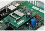
3. Use 5.5 mm socket/wrench to screw in the screws. Keep them perpendicular to the PCB as much as possible. Do not over tighten. Stop when the screw touches the PCB.
