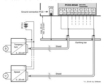
Two-wire transducers need a 24 VDC-supply in the measuring trunk.
