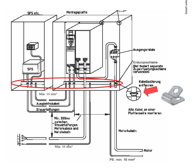
As an alternative you can use EMC compatible "panel feed-through" e. g. <u>www.distrelec.ch</u>, order no. 50 30 36 or 50 30 45)
