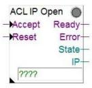
The 'ACL IP Filer' FBox allows switching on or off the IP filter function.
