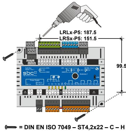
**2. DIN-RAIL MOUNTING PCD7.LRxx-P5 + MOUNTING I RM-RxC**
