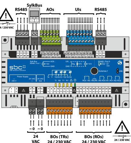
On the PCD7.LRL5-P5 the Power Supply pin 3+4 is the 24VAC power input of the controller.
