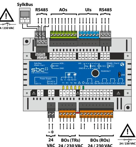
On the PCD7.LRS5-P5 the Power Supply pin 3+4 is the 24VAC power input of the controller.
