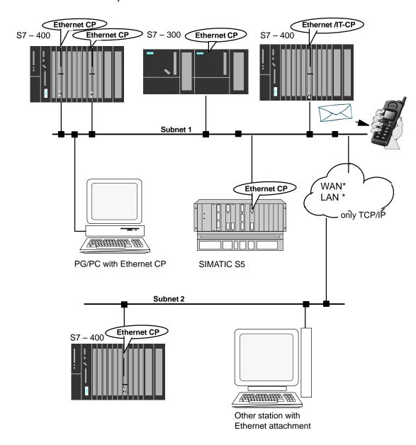
Figure 4-2 Possible Connections
