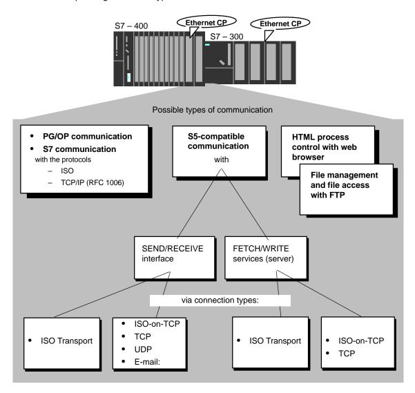
Figure 1-2 Types of Communication/Services of the Ethernet CP
