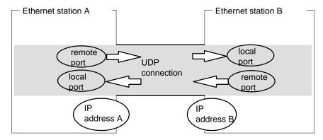
Figure 4-26 Sending and Receiving on One UDP Connection
