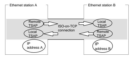
Figure 4-14 Sending and Receiving on one ISO-on-TCP Connection
