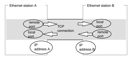
Figure 4-20 Sending and Receiving on One TCP Connection
