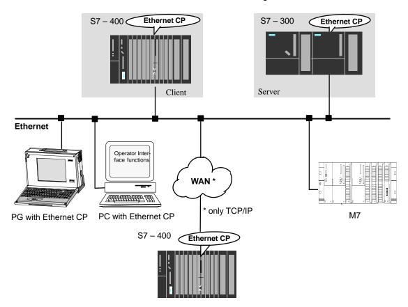
Figure 1-4 S7 Communication on Industrial Ethernet
