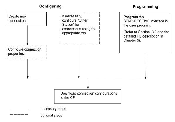
Figure 4-1 Operating Connections with the Ethernet CP
