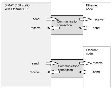
Figure 4-3 Sending and Receiving via one Communication Connection
