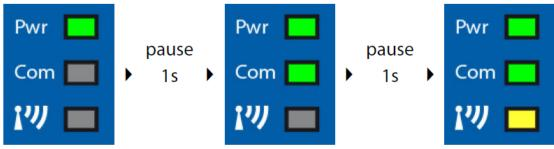
After a wrong configuration (if the user remove the config-bridge)
