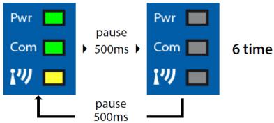
After a correct configuration (if user remove the config-bridge)
