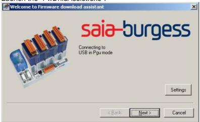
Connect the PCD3 to be updated to the PC. The possible connections are either PGU (using the programming cable PCD8.K111) or USB.
