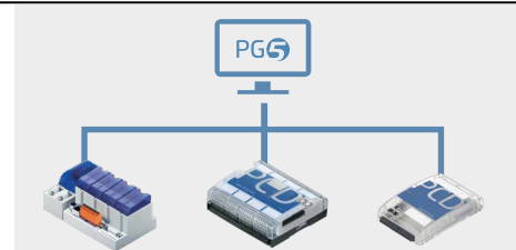
Access with the programming device via Ethernet, USB or serial interface
