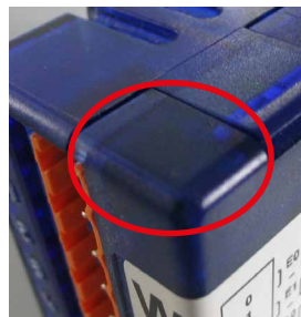
Older module housing without clip mounting option
