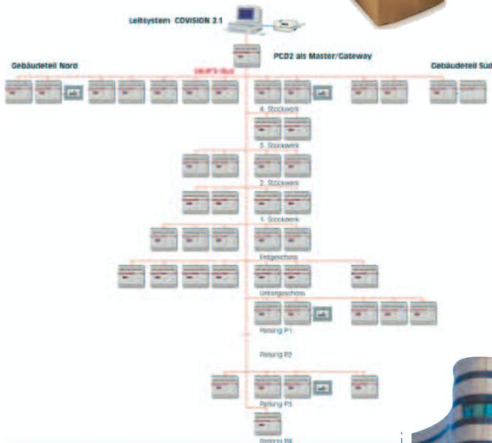
Throughout the 10 storeys each of the 45 SAIA® PCD2s controls a HEAVAC zone. They are linked to each other by the SAIA® S-Bus and also connected to the COVISION 2.1 management system via the master/gateway station. The changeover to SAIA® DDC-PLUS has resulted in large reserves of space for future expansion in the existing switch cabinets.
