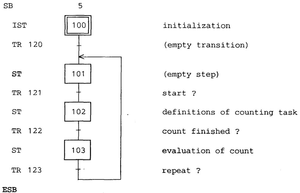
After every false transition, the program returns to the calling block (COB 0) and continues from there. All additional COBs are executed (if present). After returning to COB 0, CSB 5 (call sequential block) causes the program to re-execute all the code in the transition which was false during the previous cycle.
