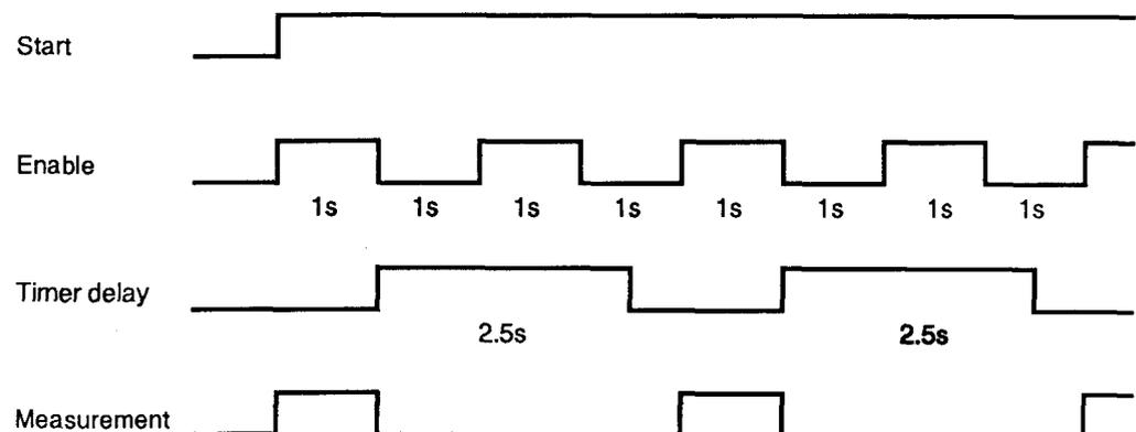
Without the delay, measurements occur whenever "Enable" is high.
