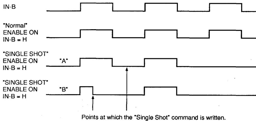
“Enable” activates counting, i.e. the enable circuit serves as a gating circuit for incoming signals to be counted. If the enable is high, signals are counted, if the enable is low, signals are not counted. (See also logic diagram in Section 4.2). The logical state of the enable circuit can be polled in the program, in order for example to allow the program to run on only after a completed count or measurement. (See Section 7.4).
