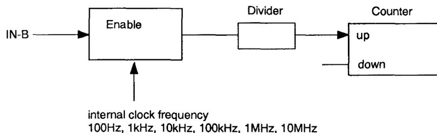
However, insertion of the divider enables clock frequencies up to 10 MHz to be used, in which case the measurement result is located partly in the counter and partly in the divider remainder.
