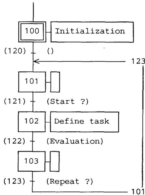
Program code is entered into individual steps and transitions in the GRAFTEC editor, or using any pure ASCII editor (not SEDIT).
