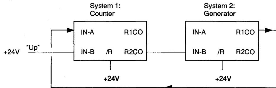
A frequency change takes place at fixed intervals of, for example, 200ms. The ramp begins at position 0. Count value is 0. Once the generator has been started, pulses with a frequency of 200Hz are output for a period of 200ms. This results in 40 pulses with a frequency of  $f_0$  for position 0.
