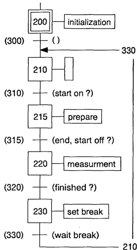
The SB containing the actual user program for the H120 module is called from COB 0 in the usual way. In addition, each time the program returns to COB 0 the display and flags are refreshed. The "Enable" flag shown at output 39 will be of particular interest in this example.
