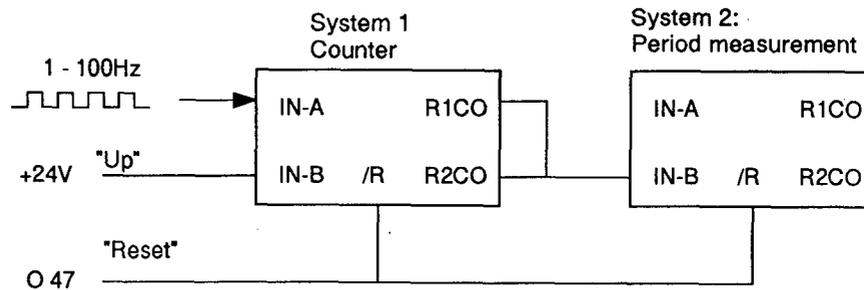
Module outputs R1CO\_1 and R2CO\_1 (open collector) are wired directly to module input INB\_2.
