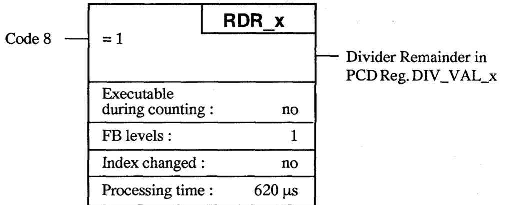
This FB reads the value of the divider remainder from the H120 module into a PCD register. This FB can only be called when counting is inactive.
