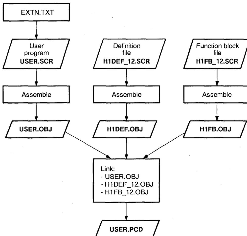
User programs for the PCD4.H120 counting and measuring module CANNOT be programmed with SAIA's "SEEDIT" editor. An ordinary ASCII text editor must be used, e.g. IBM's PE or PE2.
