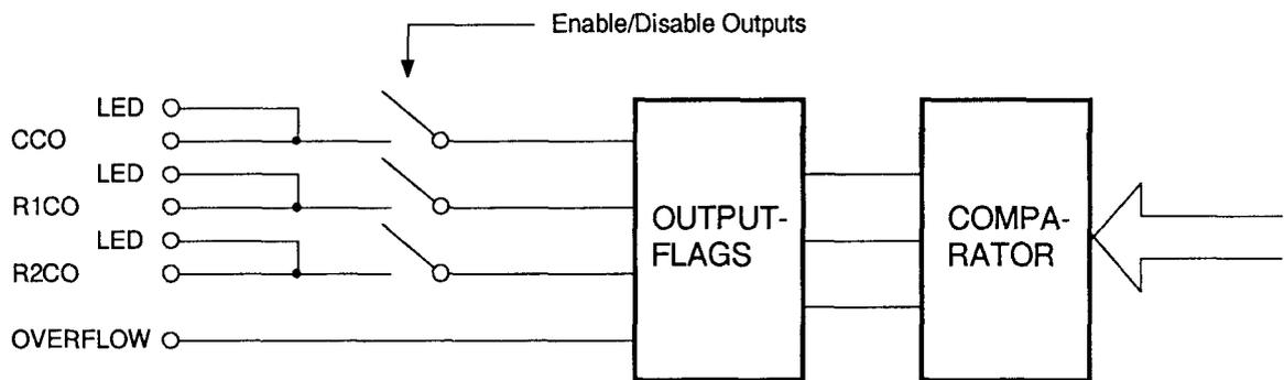
Outputs defined as unlatched remain valid until there is a (hardware) reset or until they are redefined. For example, if the definition is “Output R1CO:  $C > R1$ ”, the output flag will be high whenever the counter value exceeds the value in register 1.
