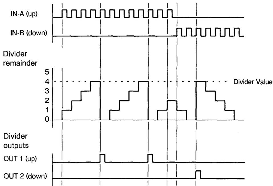
Re 3. A selected frequency from the internal clock generator can be fed into the divider, providing one of the "Divide IN-A", "Divide IN-B" or "Divide IN-A and IN-B" commands has already been executed.
