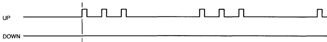
**ENABLED COUNT IN-B BETWEEN NEGATIVE EDGES**
