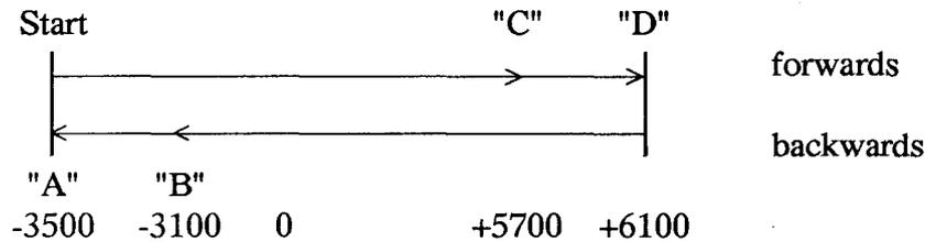
If the slide is at position "A" during power-up, the counter should be loaded with -3500 when it is switched on.
