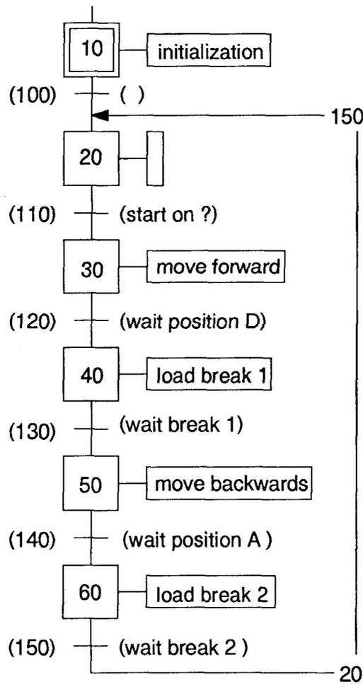
The SB is called in the usual way from COB 0. Each time the program returns to COB 0, the display and output flags are refreshed every 0.5 sec.
