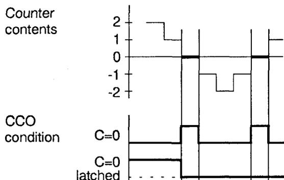
The  $C = 0$  condition sets output CCO for only as long as this condition is true. With high frequencies, this may last only a few microseconds.
