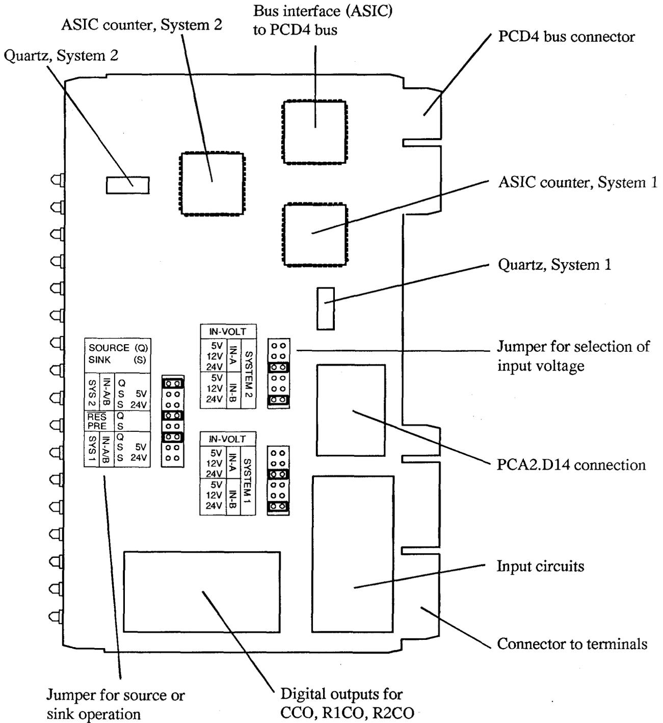
Jumper factory setting: all inputs in source operation, 24V
