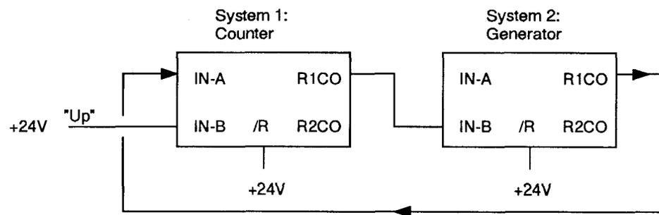
Command 250 "Count Mode: Enabled Count if IN-B = H" ensures that the generator only outputs pulses if IN-B on the generator is high. Since IN-B\_2 is connected with R1CO\_1, care must be taken that R1CO\_1 remains high until the number of pulses indicated has been reached.
