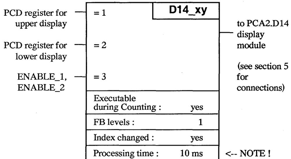
This FB can be used, for example, to write the current counter value obtained with function "RCF" (Read Counter and Flags) to the PCA2.D14 display module.
