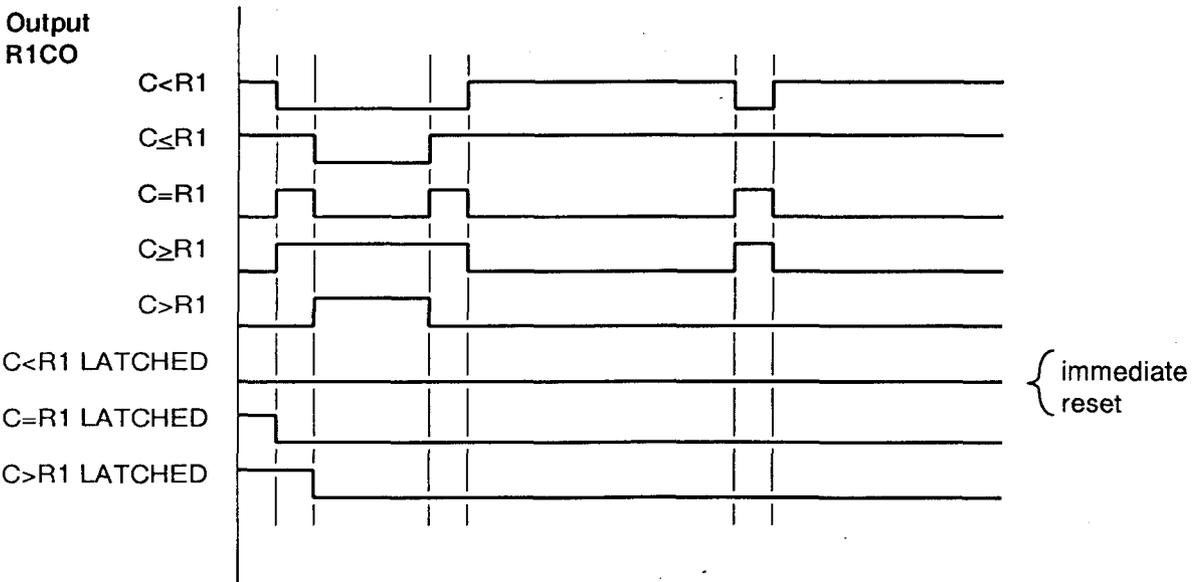
After power up, outputs “CCO”, “R1CO” and “R2CO” are inactive, i.e. all these outputs are low. After defining individual output functions, output flags are set accordingly. The outputs remain low. Only when the “Enable Output” command is executed are the output flags switched to the outputs, as the diagram shows, using the three (virtual) switches. The “Disable Outputs” command opens the switches again. The logical state of output flags is unchanged.
