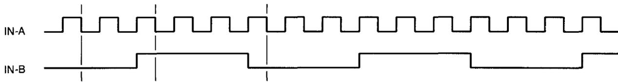
**ENABLED COUNT IN-B BETWEEN POSITIVE EDGES**
