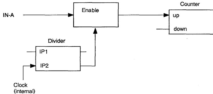
The internal clock generator, through the divider, controls the enable circuit. The enable circuit opens the time window for the duration of measurement as defined by the user program, and directs the signals arriving at input IN-A to the counter. If the time window is defined as 1 sec., after one measuring period the counter value corresponds to the frequency in Hertz.
