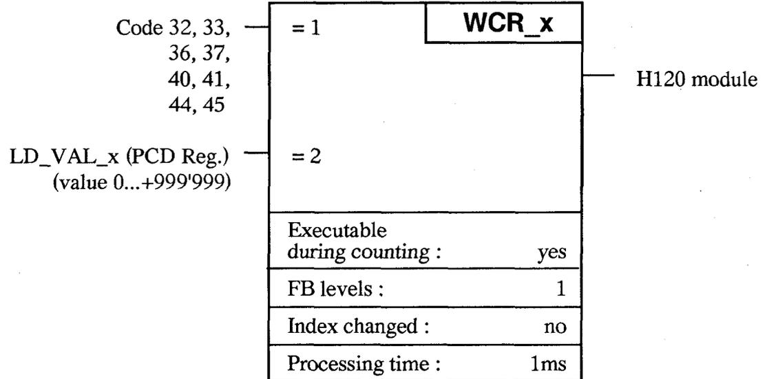
This FB writes a value 0..999'999, positive or negative, into counter register 1 or 2, or to the preset register in the H120 module.
