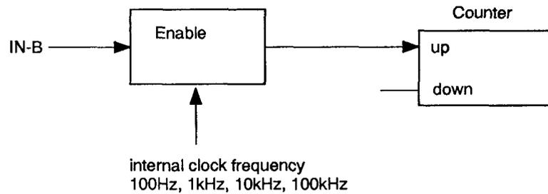
If count mode is for example "Enabled if IN-B = H", for as long as IN-B is high, the previously defined internal clock frequency is routed to the counter via the enable circuit.
