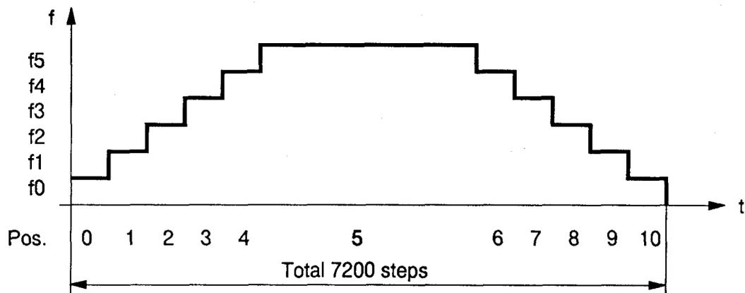
So that the ramp can be easily viewed using an oscilloscope or the model, duration of the individual positions has been set at 500 ms. In practice, this value would be substantially shorter.
