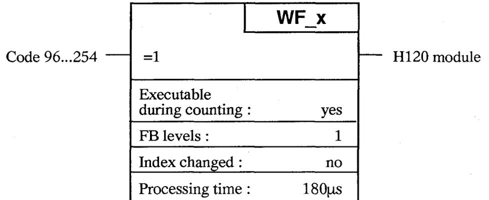
This FB writes commands to the H120 module. The 8-bit command code (96..254 decimal) is written to the H120 module's inputs 8..15.
