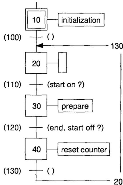
The SB containing the actual user program for the H120 module is called from COB 0 in the usual way. In addition, each time the program returns to COB 0 the display and flags are refreshed.
