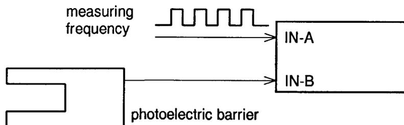
This kind of arrangement forms the basis of example "EX\_829.SRC", in which system 2 of the counting module is set up as a 10 kHz generator, so that the example can be demonstrated without needing additional devices. (The generator is discussed later in section 8.3)
