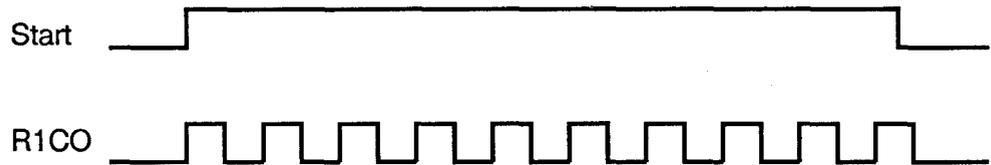
The command sequence shown at the beginning of this section is placed in the user program. Once this command sequence is executed, the counting module works independently as a pulse generator, with the values given. This was already done in example “EX\_829”.
