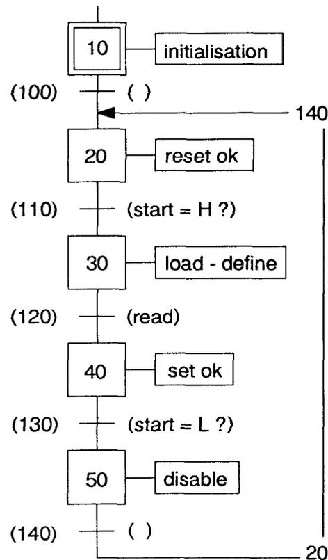
The SB is called from COB 0 by the user program. Each time the program returns to COB 0 the display and output flags are refreshed every 0.5 sec.
