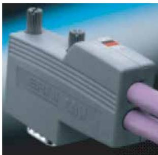
Other manufacturers like Delconec or FCT also provide CAN bus couplers. According to ISO 11898 Norm, Cable line impedance must be 120 Ω. For CAN cabling the use of twisted pair cable (2x2) having an impedance of 108...132 Ω is recommended.
