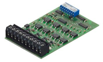
Low cost output module with 8 transistor outputs 5 ... 500 mA, without short circuit protection. For non-isolated circuits in the voltage range 5 ... 32 VDC.
