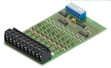
Low-cost input module for source or sink operation with 8 inputs, electrically connected. Suitable for most electronic and electromechanical switching elements at 12 VDC.
